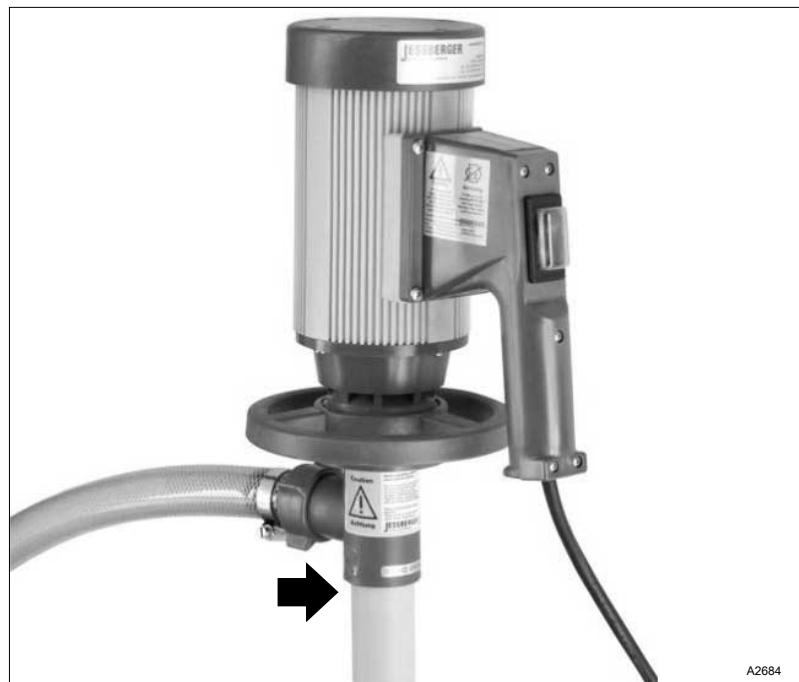
Fig. 6: Lip (arrow) of the outlet nozzle.
