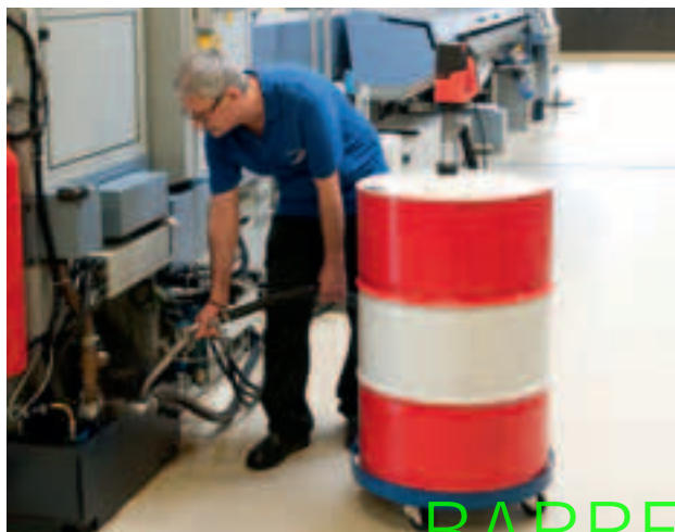
Filling a system with hydraulic oil (F 430 AL).
